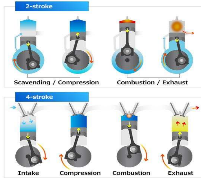
Figure 2.3: Two-Stroke and Four-Stroke Engine Cycles (Herold et al., 2011).
