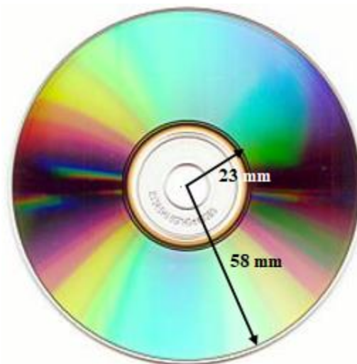
Fig. 2: A compact disk track
