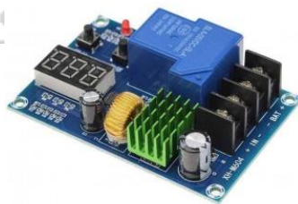
Figure 2.26: Charge Control Module
