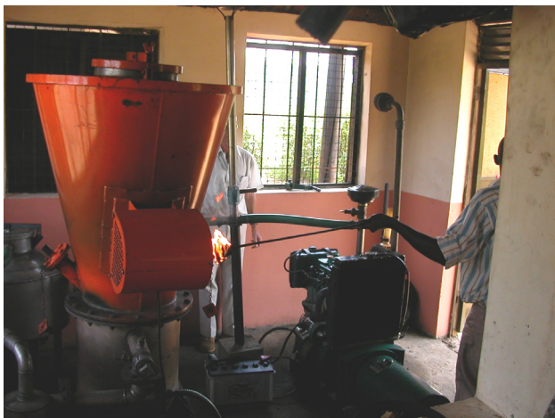
Figure 2: 10 kW dual fuel mode gasifier for electricity production.
