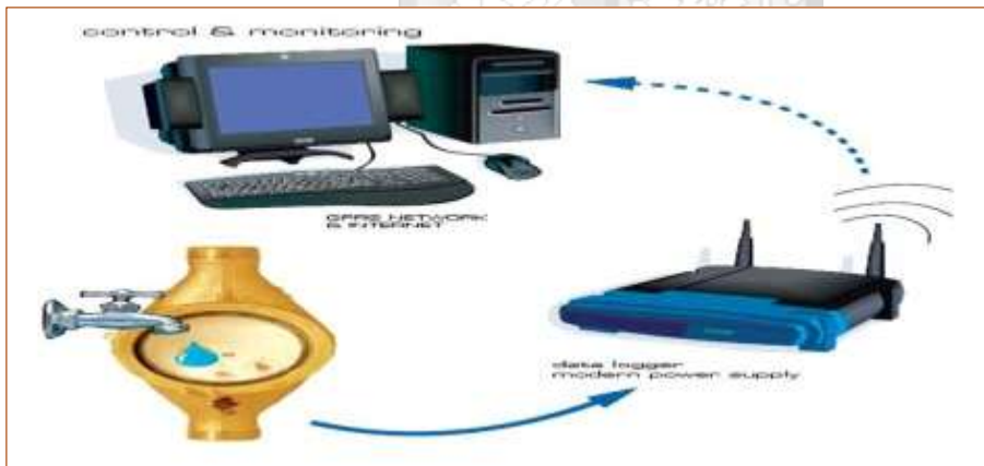
Figure 2. 14: Typical smart meter water set up (Davidson et al., 2016)
