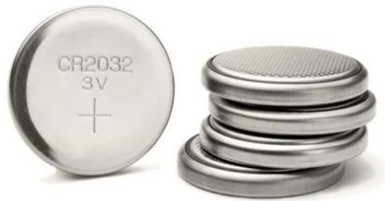
Figure 2. 2: Coin Cells (Idelah, 2020)
