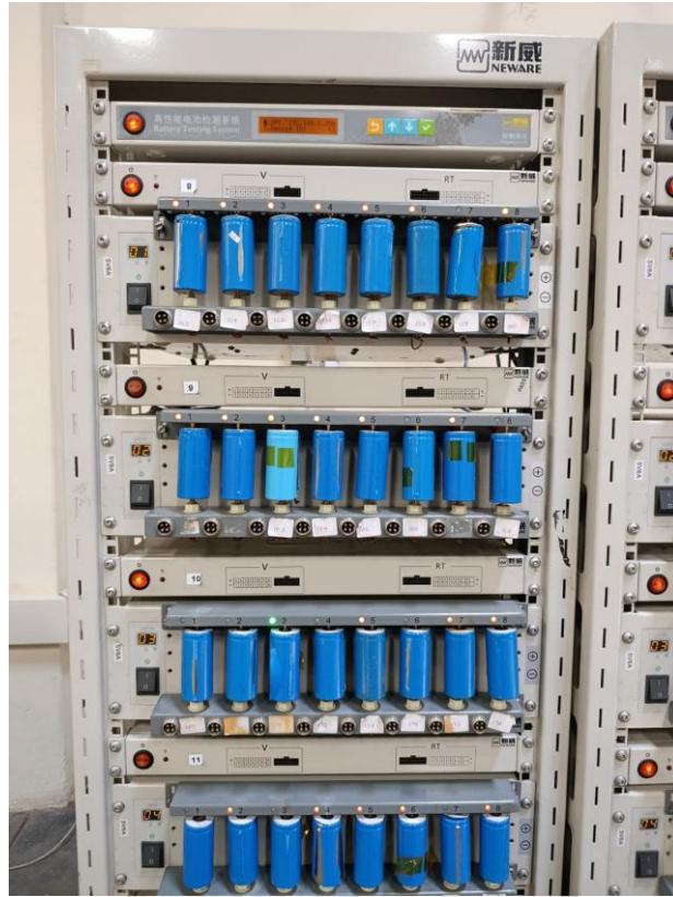
Figure 3. 1: Neware CT-4008T-5V6A-S1 Cell Tester
