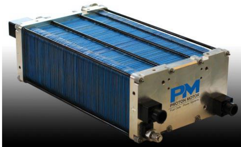
Figure 2.8: A 96-cell PEMFC stack, which is water-cooled and capable of generating up to 8.4 kW while weighing 1.4 kg. (Source: Proton Motor GmbH)
