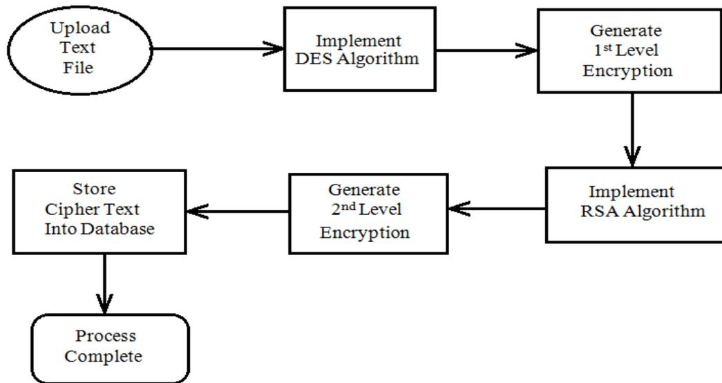
**Figure 2: 6: Block Diagram of Multilevel Encryption (Khan & Tuteja, 2015).**
