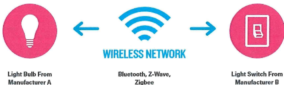
Figure 2.2: Device-to-device model (The Internet Society, 2015)
