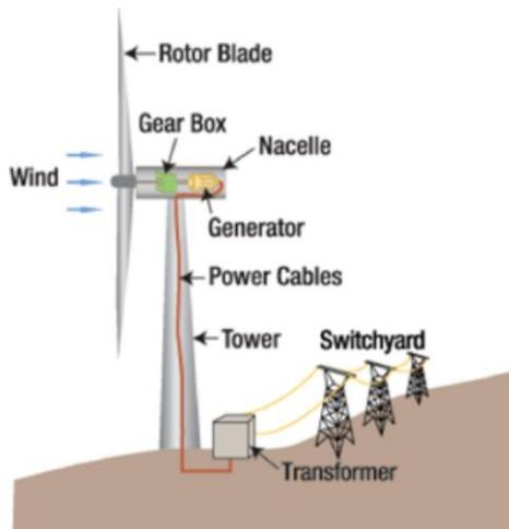
Fig.1: Main parts of a modern wind turbine
