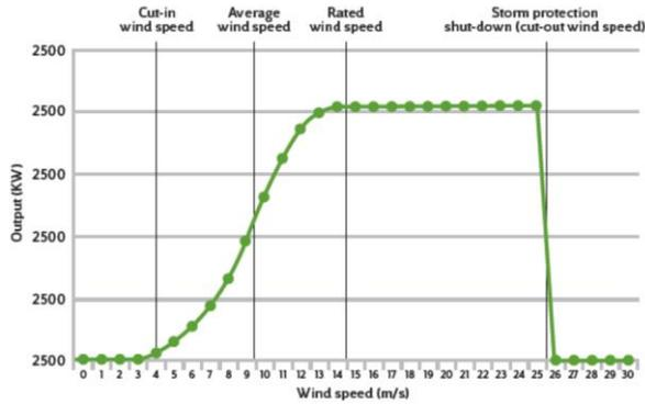
Fig. 4: Typical power curve of a 2.5MW turbine
