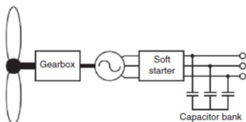
Fig. 8: Power electronics in modern wind turbine
