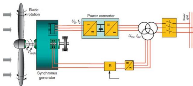
Fig. 7: Direct drive synchronous generator
