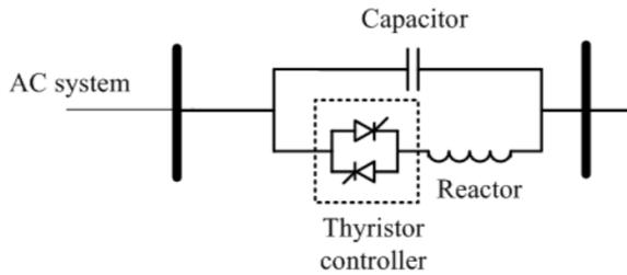
Fig. 11: TCSC schematic representation
