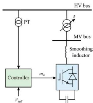
Fig. 10: STATCOM schematic representation
