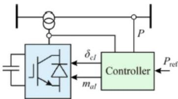
Fig. 12: SSSC schematic representation
