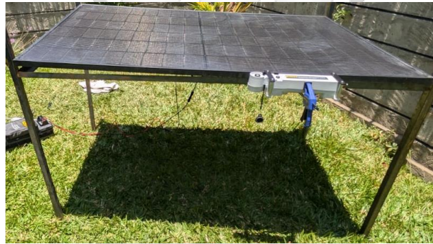
Figure 4.6: Bifacial PV Module Mounted on a Grass Surface
