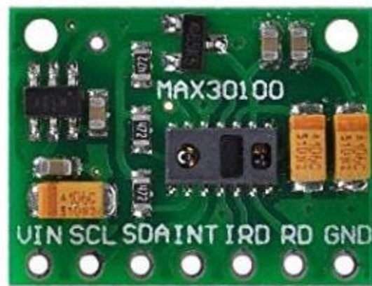
Figure 5. 2 MAX30100 Sensor (Hema et al., n.d.)
