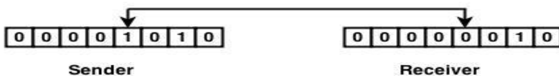
Fig: 2.3.1(a). Single bit error illustrating the transformation of 1 to 0, from sender to receiver.
