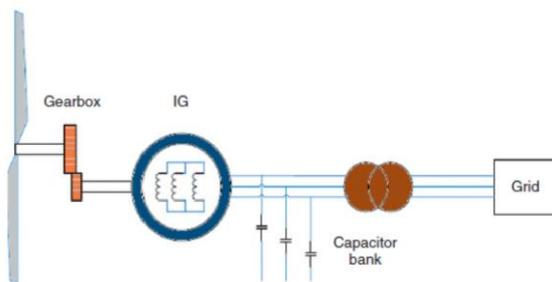
Fig. 5: Squirrel cage induction generator
