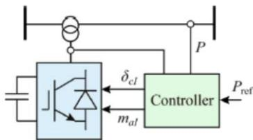
Fig. 12: SSSC schematic representation
