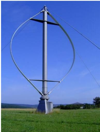
Fig. 3: Vertical axis wind turbine
