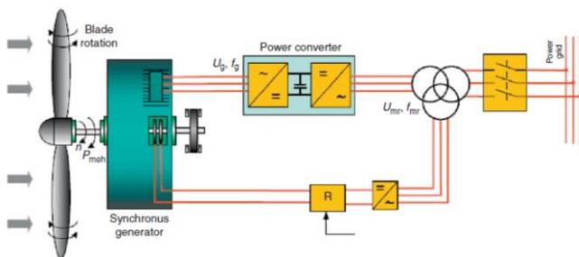
Fig. 7: Direct drive synchronous generator
