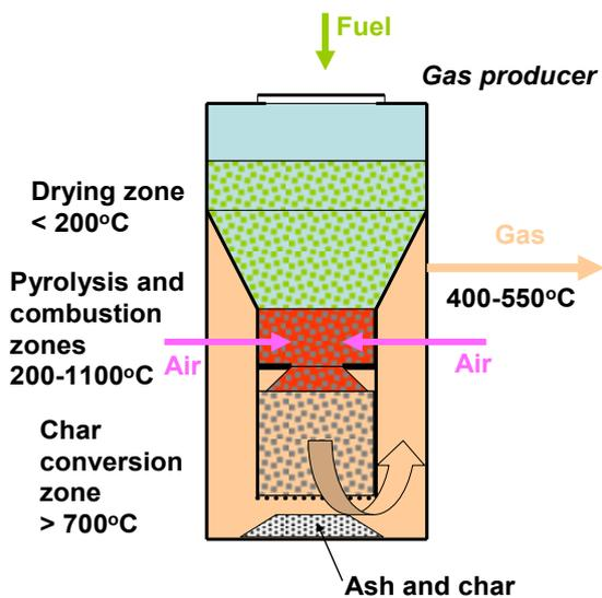
Figure 2. Principle of downdraft gas producer with throat
